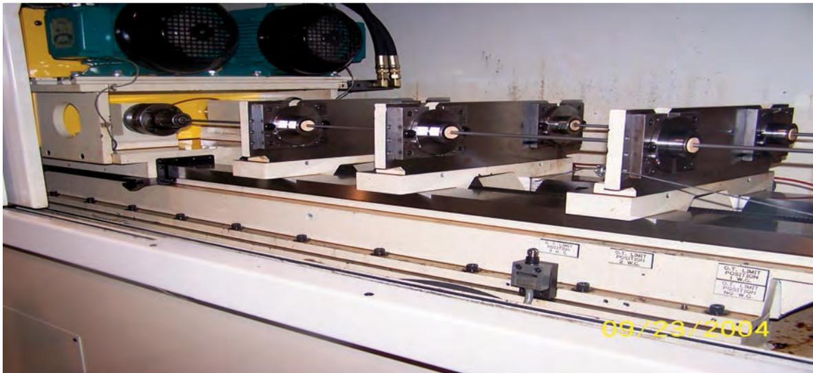
Whip Guide Stabilizers mounted on whip guide supports.
