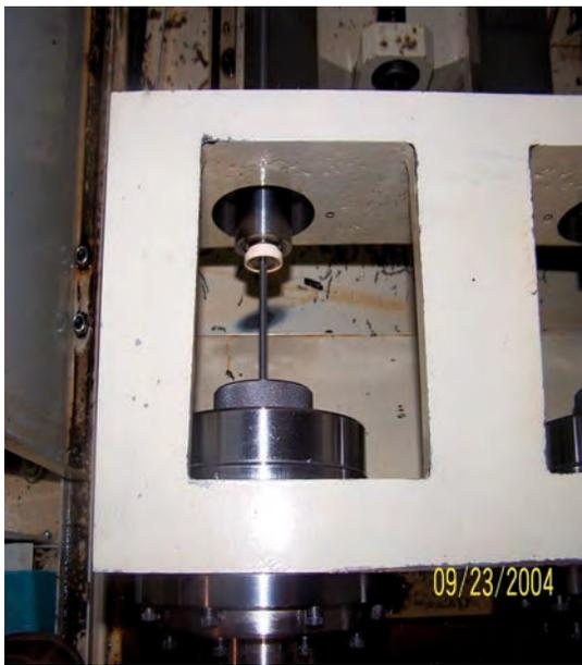
Chip box with Gadget Snap On Chip Deflector and Whip Guide Stabilizer. Drill straighter and faster with the whip guide Stabilizers and Adaptors.
